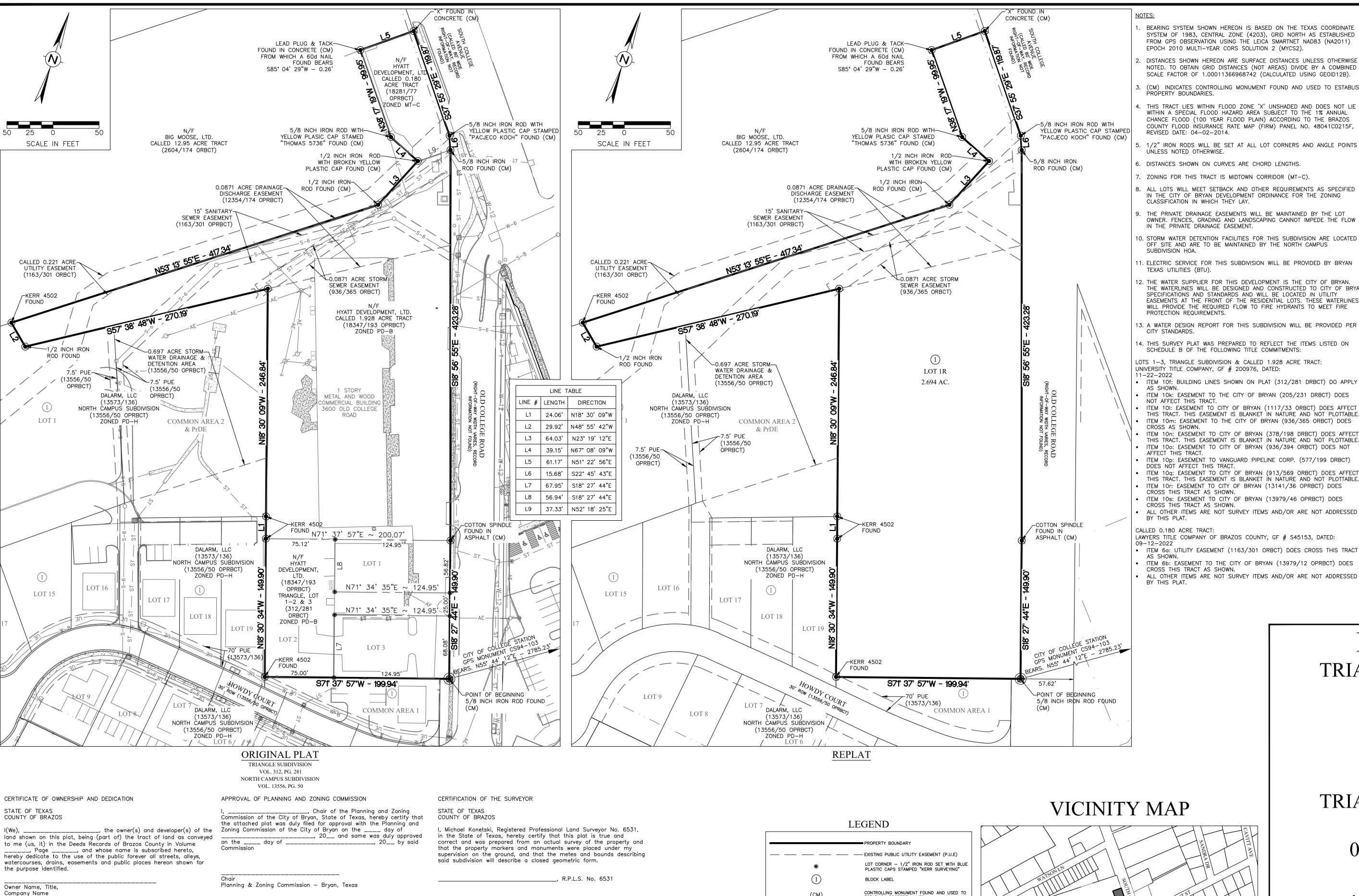
DISTANCES SHOWN HEREON ARE SURFACE DISTANCES UNLESS OTHERWISE NOTED. TO OBTAIN GRID DISTANCES (NOT AREAS) DIVIDE BY A COMBINED SCALE FACTOR OF 1.00011366968742 (CALCULATED USING GEOID12B).
